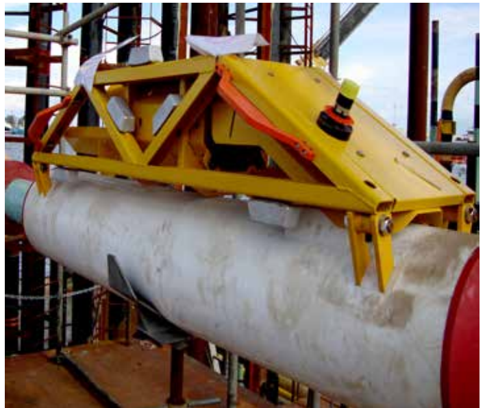
Figure 4. Subsea CEM with transducers installed under insulation. The sensor electronics are located in a ROV retrievable canister.
